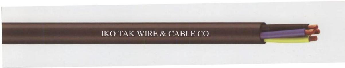
Conductor: group 5 annealed copper (flexible) as per ISIRI 3084 or 60228 IEC standard. Insulator: PVC mixture of PVC/D type. String placement manner: (1) round cable: strings are twisted together (2) flat cable: strings are placed in parallel. Coating: PVC mixture of PVC/ST5 type. Coating color is normally black. Standard: ISIRI (607) 53, 60227
