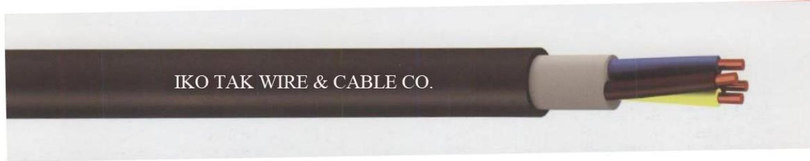
Conductor: group 1 annealed copper (single string): or group 2 (regularly twisted) as per ISIRI 3084 or 60228 IEC standard. Insulator: PVC mixture of PVC/C type. String placement manner: strings are twisted together; middle coating: the twisted strings and extruded and coated with PVC mixtures. Coating: PVC mixture of PVC/ST4 type. Coating color is normally black or white. Standard: ISIRI (607) 10, 60227 IEC 10 with 300-500V nominal voltage
