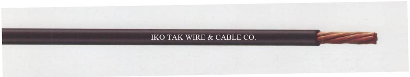
Conductor: annealed copper with max. dia. 0.21mm. Separator: PE tape covering the conductor. Insulator: TPR mixture with minimum tension strength of 12.5 N/mm<sup>2</sup>, THK: 2.4~3.2mm. Standard: 245 IEC 81 [ISIRI (1926) 81]
