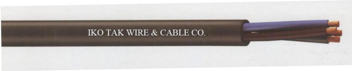
Conductor: group 5 annealed copper (flexible) as per ISIRI 3084 or 60228 IEC standard. Insulator: PVC mixture of PVC/D type. String placement manner: (1) round
