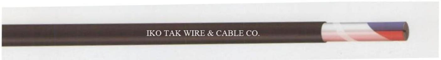
Conductor: group 1 annealed copper (single string): or group 2 (regularly twisted) as per ISIRI 3084 or 60228 IEC standard. Insulator: PVC mixture of PVC/C type. Standard: ISIRI 3569, IEC 60520 with 600-1000V nominal voltage
