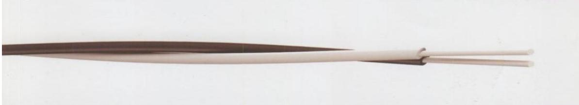
Conductor: tinned single string annealed copper. Insulator: PVC mixture with quire high quality. Coloration of insulators is black and white for doubles and black, and black, white and green for triples. Strings twisting manner: the strings are twisted together in doubles or triples with 30mm twisting length. Standard: VDE 0815 or TCI (Telecommunications Company of Iran) specifications.
