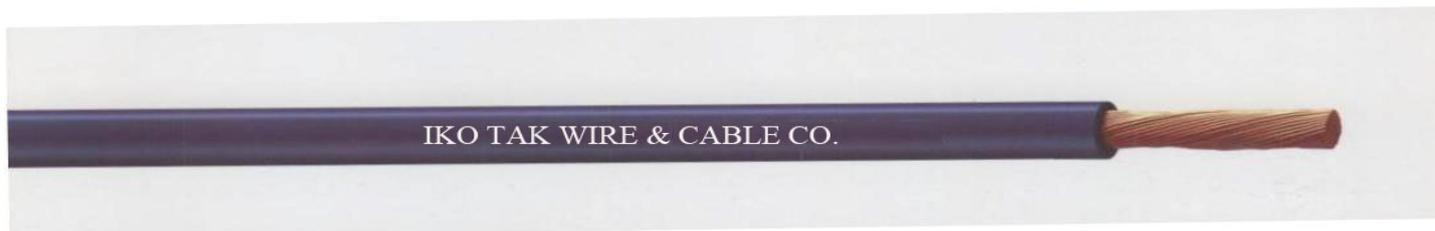
Conductor: group 5 annealed copper (flexible) as per ISIRI 3084 or 60228 IEC standard. Insulator: PVC mixture of PVC/C type. Standard: ISIRI (607) 02, 60227 IEC 02 for
