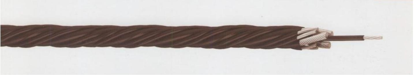
Twisted and compressed (ACC) as per ASTM B231. 6-string cables: null conductor and messenger: alloy aluminum (AAAC) 1. Messenger: 7 string twisted high carbon galvanized steel strings. Insulator: black linked cross polyethylene XLPE for phase string, lighting and null and black high dense polyethylene HDPE for messenger string. Standard: TAVANIR specifications
