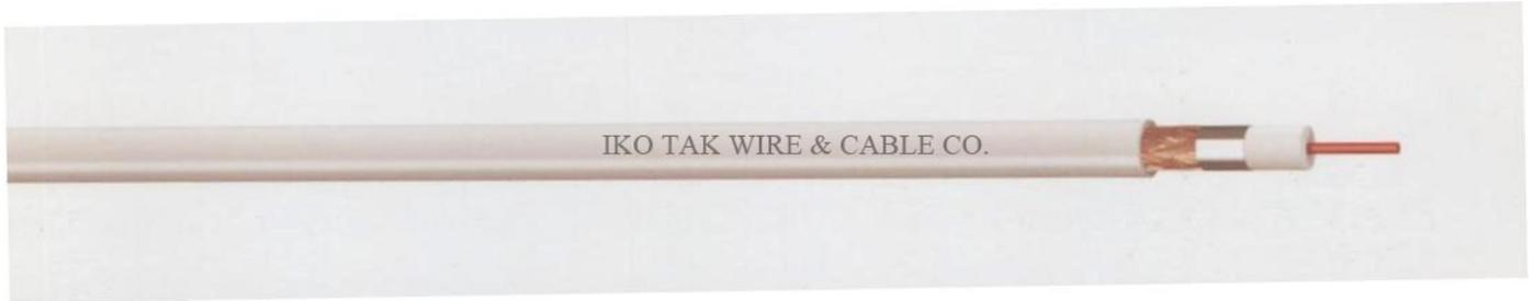
Conductor: single string or regularly twisted, simple or tinned annealed copper. Insulator: PE mixture in solid or fume manner. Simple or tinned simple copper wire in woven manner; Coating: special PVC mixture. Standard: JIS 3501
