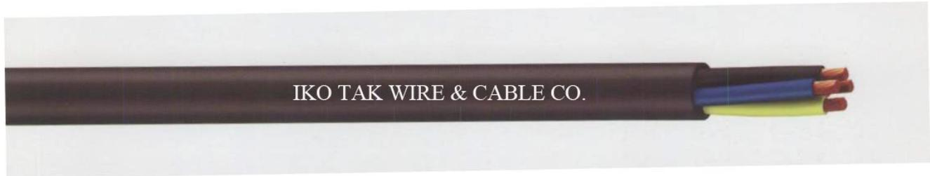
Conductor: annealed copper group 5 (flexible) as per IEC 60228 or ISIRI 3084 standard, insulator: PVC mixture of PVC/D type. Strings manner of placement: the strings are twisted together with twisting length specified in the standard. Coating: PVC mixture of PVC/ST5 type. Coating coloration is normally black. Standard: ISIRI (607) C71 or IEC 60227 71C with 450/750 V nominal voltage.
