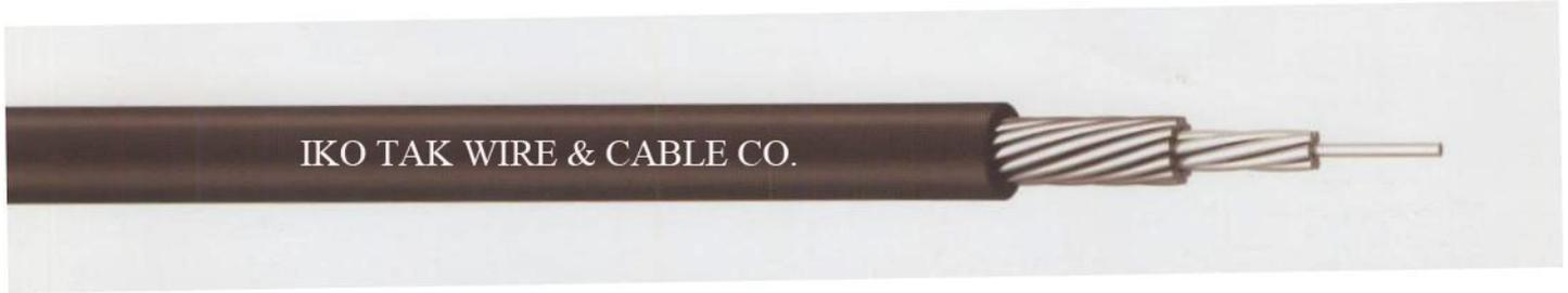
Conductor: group 5 annealed copper (flexible) as per ISIRI 3084 or 60228 IEC standard. Insulator: PVC mixture of PVC/D type. String placement manner: (1) round cable: strings are twisted together (2) flat cable: strings are placed in parallel. Coating: PVC mixture of PVC/ST5 type. Coating color is normally black. Standard: ISIRI (607) 53, 60227 IEC 53 with 300-500V nominal voltage.
